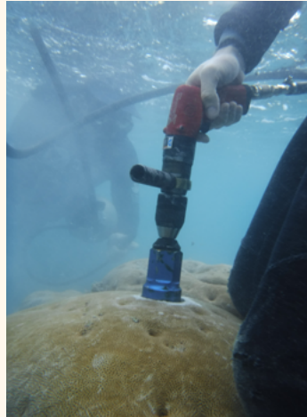
The pneumatic underwater drill, first purchase made with Serrapilheira grant funds © Personal file
